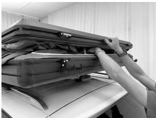
5.8) Push all fabric as well as the pull strap into the shell.
