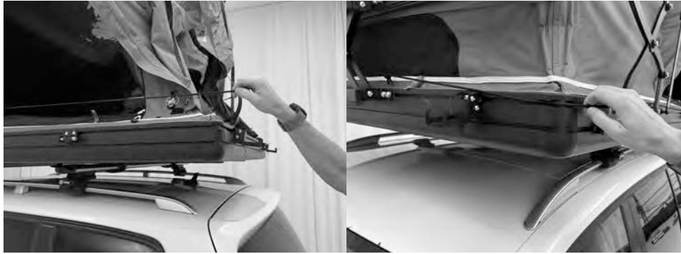
4.3) Move the elastic cord from the fabric and hook it to the corners of the shell. Repeat for all four corner, so the elastic cord is completely free from the fabric.
