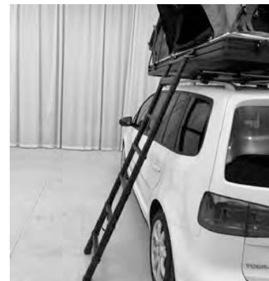
4.7) Attach ladder to ladder brackets. Open the brackets by pulling on the spring loaded knob. Ensure that brackets are fully closed after attaching the ladder.
