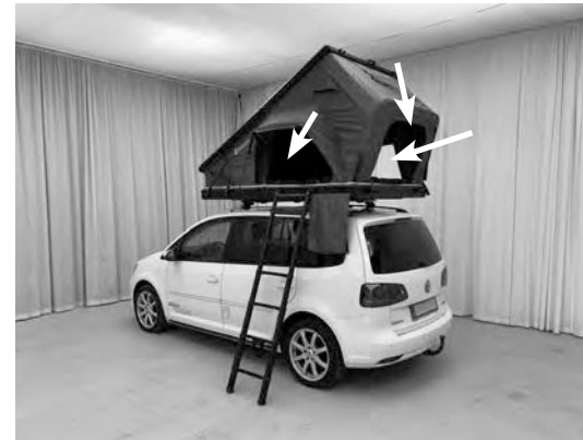
2.8) Install the ladder brackets at your chosen door location. The ladder can be installed on both sides as well as on the rear of the tent.
