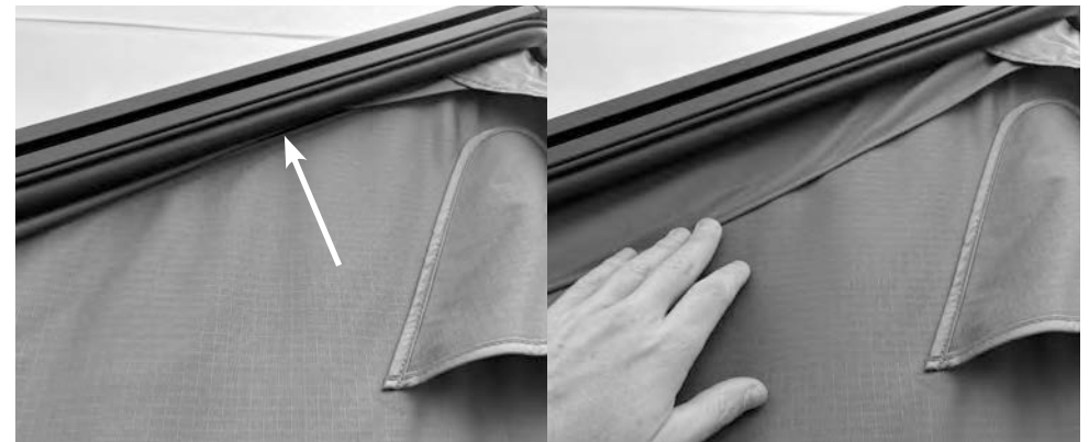
4.13) Sometimes it can happen that the flap shown above becomes stuck under the seal on the upper shell. If this happens pull it free to ensure full protection in all weather conditions.
