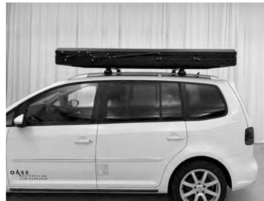
5.11) Test that the tent is still securely fastened to the vehicle before driving away. Re-tighten if needed.
