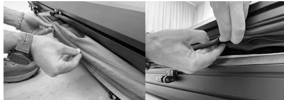
5.9) Tuck the canopy poles up behind the rubber seal on the upper shell of the tent.
