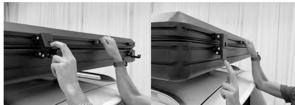
5.10) Close the latches starting on the rear of the tent. Use the handle to assist. Ensure all four latches are fully closed, and that no fabric is jammed between the rubber seals of the upper and lower shells.
