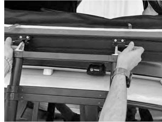
5.3) Remove the ladder by pulling on the knobs of the ladder brackets.
