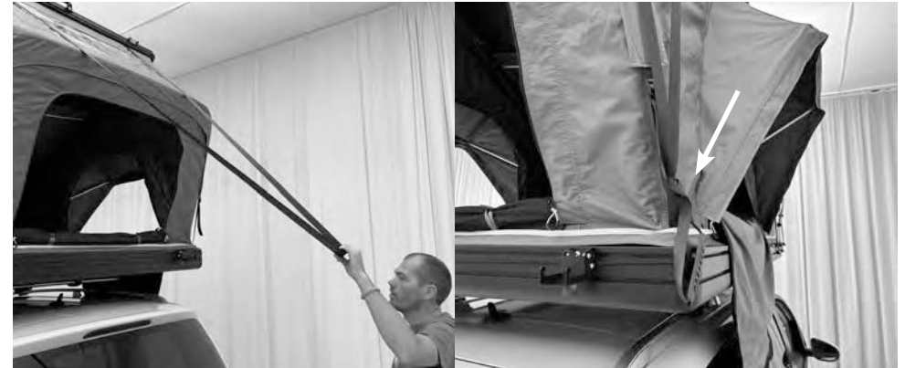
4.12) Tie the pull strap to the corner of the fly, to prevent it from moving in the wind.
