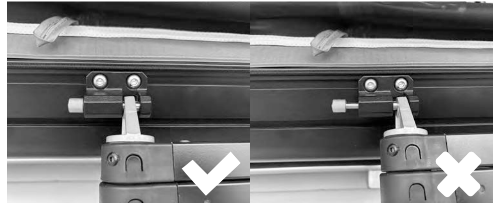
4.7) Attach ladder to ladder brackets. Open the brackets by pulling on the spring loaded knob. Ensure that brackets are fully closed after attaching the ladder.
