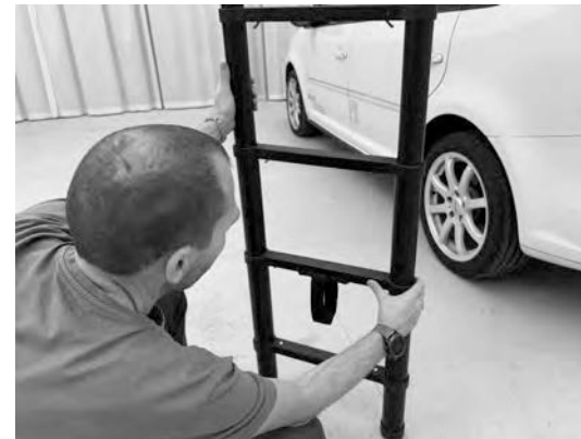
5.4) Close the ladder. Unlock one sliding button at a time while holding the stile of the upright ladder with your other hand (so it does not collapse by its own weight).
