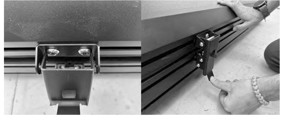
2.7) Flip the "latch lower part" up and into the "latch upper part". Center the upper part in relation to the lower part. Tighten the bolts on the upper part. Re-assemble the latch upper part fully, and test the function of the latch. Repeat for all four corners of the tent.
