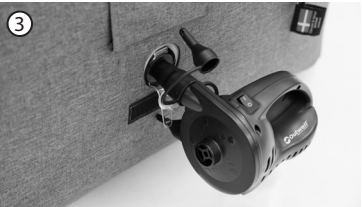
When fully inflated seal valve by pushing in the pump nozzle. This will seal the internal stopper and keep air from escaping while closing cap.
