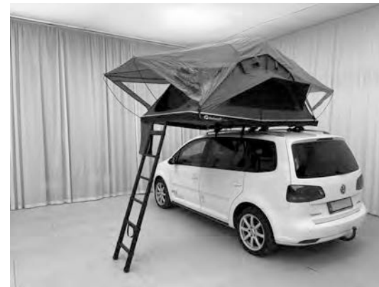
4.11) Set ladder length and angle to support the tent. Observe the ladder angle limitations of 65°-75°. Ensure ladder rungs are locked from the bottom and up. E.g. if only 5 rungs are needed, it must be the two top rungs that remain unlocked.
