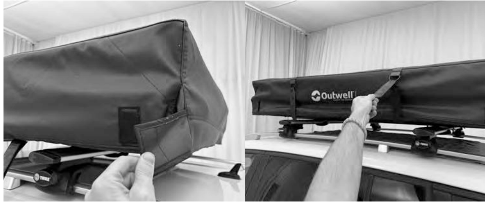
5.10) Close the two velcro tabs on the front of the tent. Bring the two long straps over the tent, and secure them with the velcro loops.
