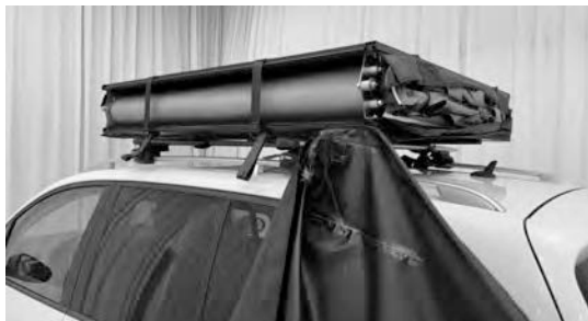
5.7) Slide the beading of the transport cover into the c-channel on the tent. Put the transport cover in place.
