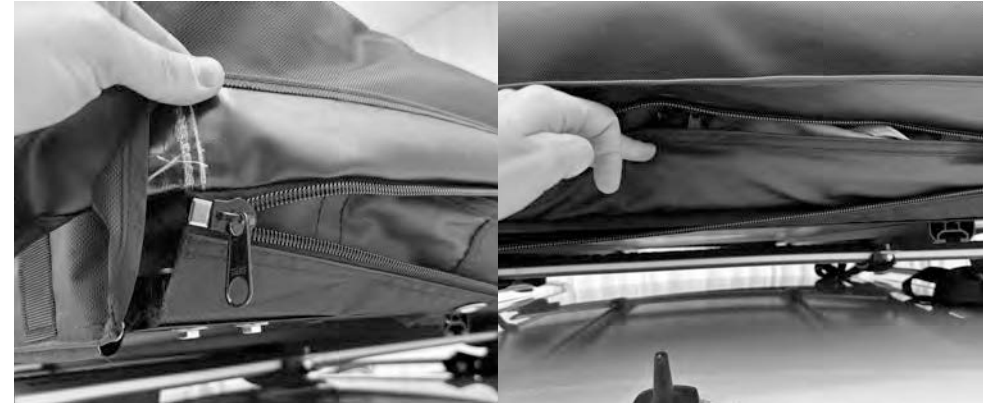
5.8) Locate the zipper ends and zip the transport cover to the tent. Pull up the fabric behind the zipper, to avoid the zipping into the fabric edge.
