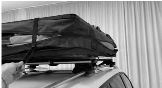
5.6) Close the two velcro straps on the rear corners of the tent.
