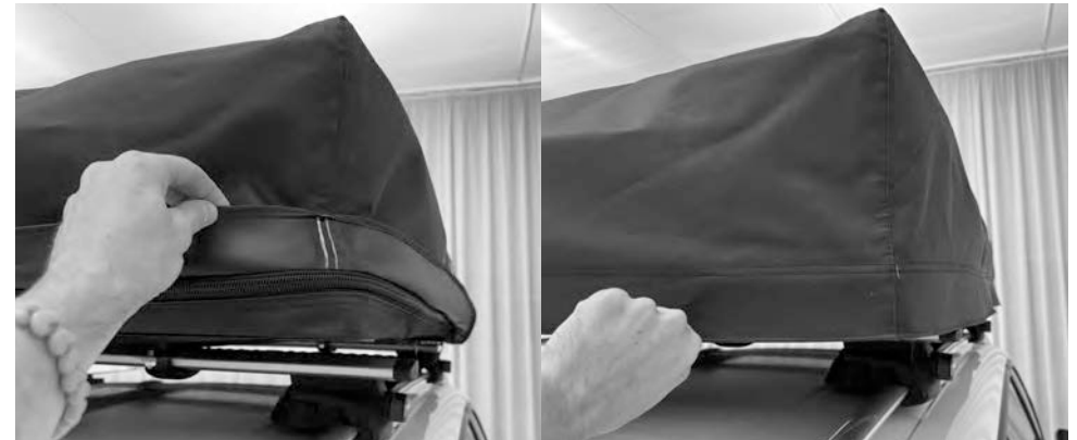
5.9) Fold the edges of the transport cover back down.
