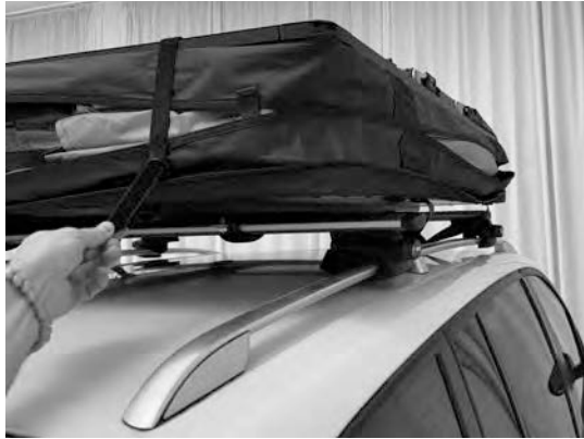
4.6) Open the two velcro straps on the rear corners of the tent.
