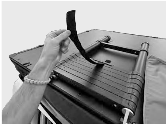
4.7) Undo the velcro retainer strap on the ladder.
