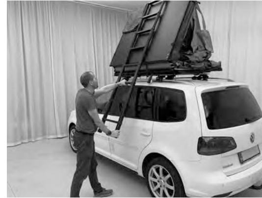
4.9) Grab the bottom of the ladder. Pull the ladder out fully. Observe that all rungs are locked.
