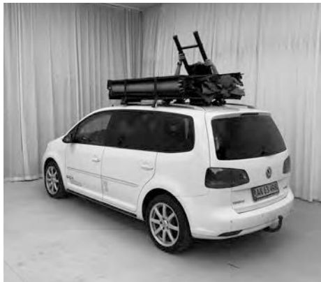
4.8) Extend the first three sections of the ladder, so the bottom of the ladder can be reached from the other side.
